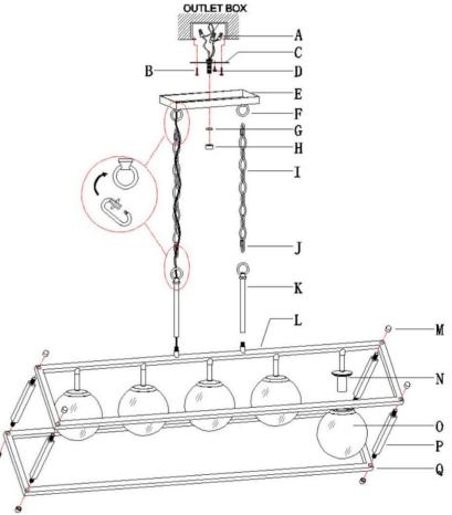
Step A1: Secure threaded pipes (P) onto lower frame (Q) and fixture body (L) with lock nuts (M).
