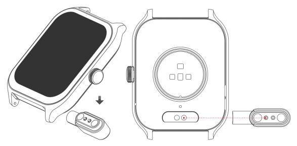
Long press the side button for 3 seconds or plug in the Magnetic charging cable to charge the Smart Watch.
