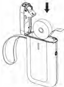
❸ Consumable installation
