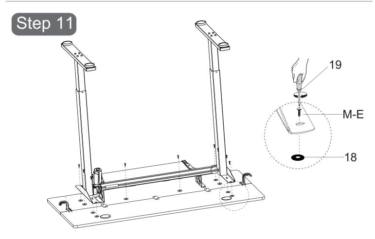
Use screwdriver(19), secure the Leg part to the Boards (7a&7b) with Screws (M-E)\*10. Please align the Silicone Sheet (18)\*10.
