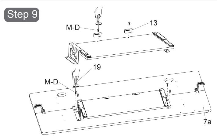
Use screwdriver(19), with Screws (M-D)\*2, Attach the keyboard retainer (13) \*2 to the drawer.
