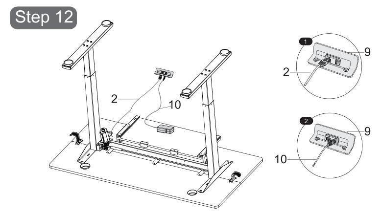
As shown, connect the motor at the Left Leg (2), Hand Controller (9) and Power Supply (10) in turn.
