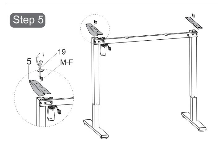
Use screwdriver (19), install Side Plate (5)\*2 on each side of the Legs (2&3) with Screws (M-F)\*4.
