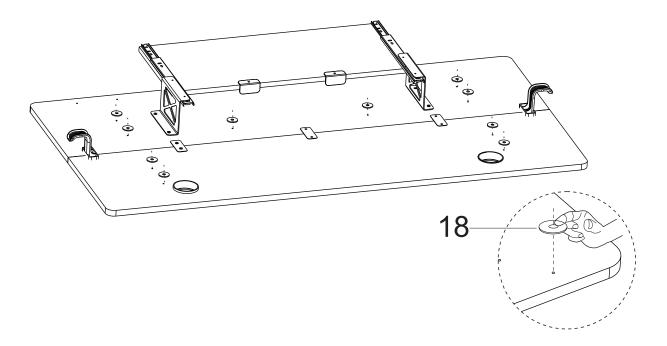
Fix Silicone Sheet (18)\*10 to the corresponding hole position on the Boards (7a&7b).
