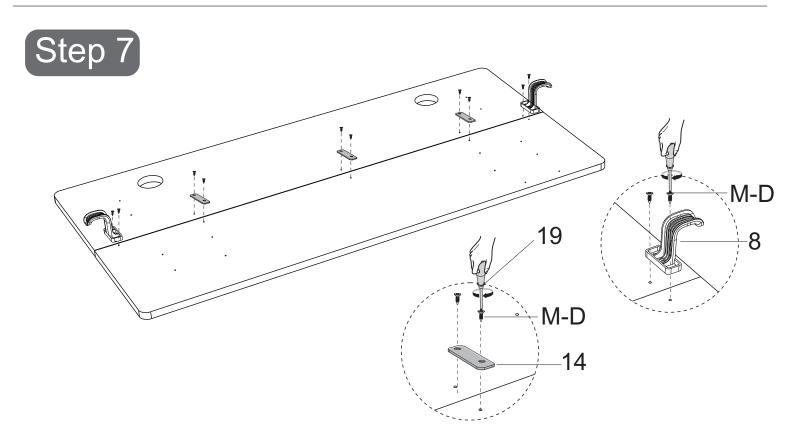
Fix Boards (7a&7b) with Wooden Pin (16)\*4. Use screwdriver(19), with Screws (M-D)\*10, install Desk Connection Plate (14)\*3 to the middle of the Boards, and Desk Connection Hook (8)\*2 to both sides of the Boards.
