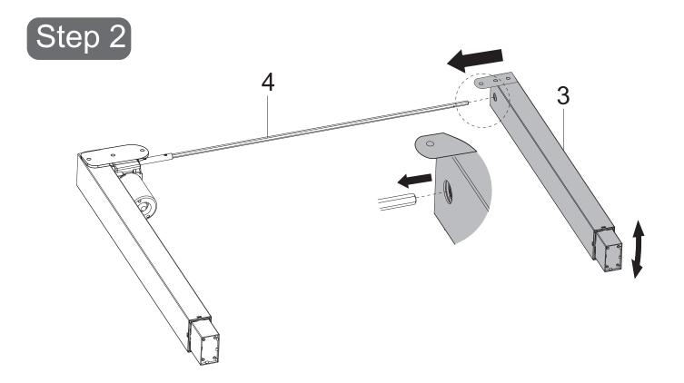
Insert the drive rod (4) into the hole in the right leg (3). If it is not possible to insert, please rotate the right leg (3) slightly until the inner hexagon matches.
