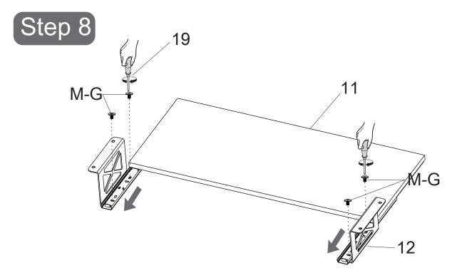
Pull out the orbitals completely (11). Use screwdriver(19), with Screws (M-G)\*4, Attach the drawer connector to the track
