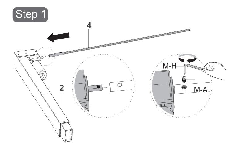
Align the holes of Left Leg (2) and Drive Rod (4), Using Wrench(M-H) to secure both with Screw (M-A).
