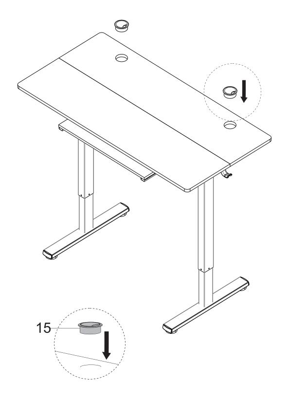
Insert Cable Hole Cover (15)\*2 into the hole in the Board (7b).
