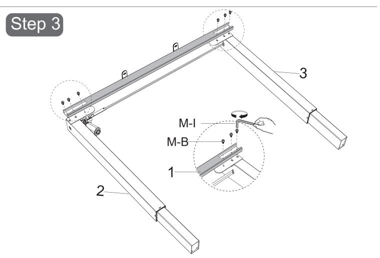
As shown, use Wrench (M-I), install Beam (1) to the Legs (2&3) with Screws (M-B)\*6.
