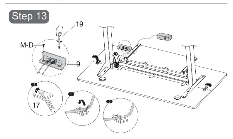
Using screwdriver(19), install Hand Controller (9) to the Board (7a) with Screws (M-D)\*2. Secure the connecting cable with Cable Clip (17)\*2 and glue it to the bottom of the Board.
