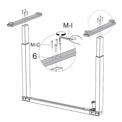
Using Wrench(M-I), install Leg Base (6)\*2 to the Legs (2&3) respectively with Screws (M-C)\*8.
