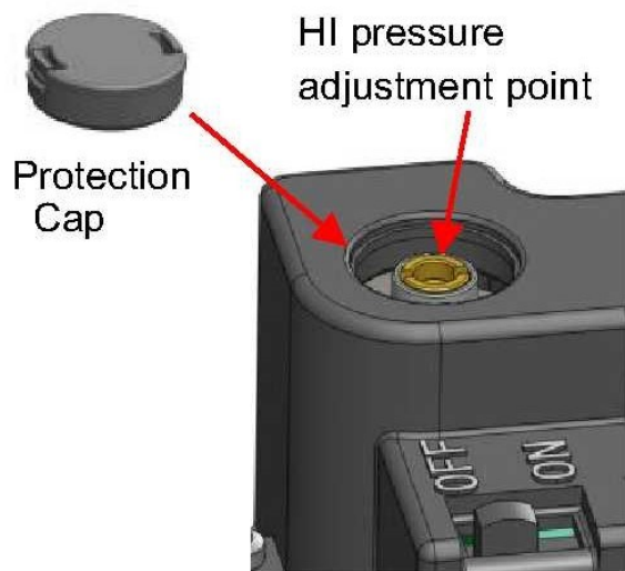
Figure 21. Sanhua gas valve high pressure adjustment
