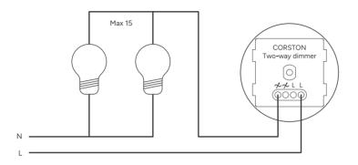
Some lamps may exhibit unexpected performance characteristics when cold. Dimming performance should improve after the lamp warms up. If the lamp begins to flicker or there are dimming issues, the dimmer may need to be changed from TE to LE mode or vice versa.
