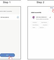
3. When the LED strip not blink after powered on. Please press the function button for over 5 seconds, then the light turn to quick flash, enter into the APP and choose to add all the device in the corresponding room in the APP. Enter into the interface of adding lighting device and match the LED strip
