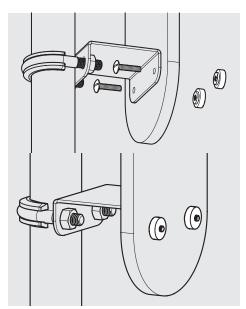
Secure the bottom section of the Placard Board with the Plastic Screws & Nuts. Installation now complete.
