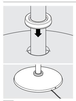
With the Cover on the ground, locate & fit the Rubber Collar.
