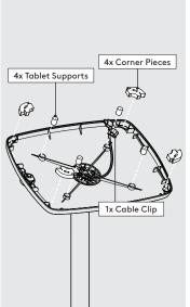
Install the Tablet Setup Kit. Each kit is specific per Tablet & Case.
