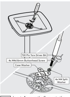
Locate & secure the Case onto the Floorstanding Pole as shown. Tighten by hand.
