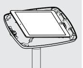
Install the Tablet into the Case & connect to Power Cable.
