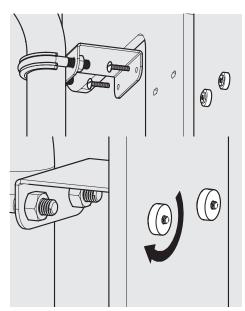
Locate the Placard Board to the Bracket Mount. Secure with the supplied Plastic Screws & Nuts.
