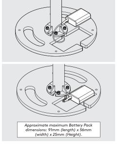
**9.2** If installing a Battery Pack, connect the Power Cable & locate into the Base.
