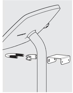
Locate the top Bracket Mount & **A2** Mount Bolt to Floorstanding pole.
