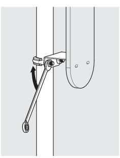
Locate & secure the bottom Bracket A6 Mount & Mount Bolt. Tighten the nuts
