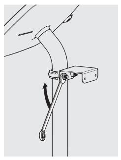
Secure the Bracket Mount & Mount Bolt to the Floorstanding Pole with the supplied Nuts. Tighten evenly.
