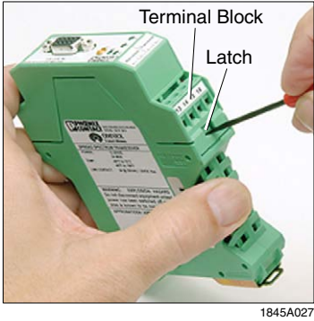
Figure 3-4. Opening Housing to Access DIP Switches
