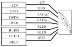
The device has the function of Wiegand signal input. It supports to connect with an independent card reader.
