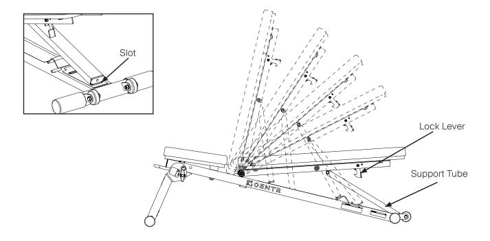
Swivel lock lever under pad to release back pad. Raise the head end of the pad so the free end of the suport tube slips into a slot for a desired position. Before use, make sure the support tube is secure in a slot. Five degrees are available.
