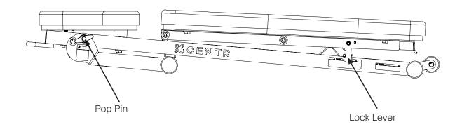
Pull pop pin to unfold or fold leg. Make sure hands are clear of pivot area. Make sure pop pin is fully engaged in locking holes after each adjustment.
