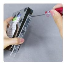
**02.** Connect the HDD guard to a SATA HDD as shown on the picture. Fasten the screws.
