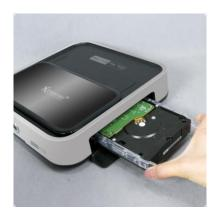
**Q3.** As shown here, slowly and carefully push the HDD guard together with the SATA HDD into the main body of iXtreamer
