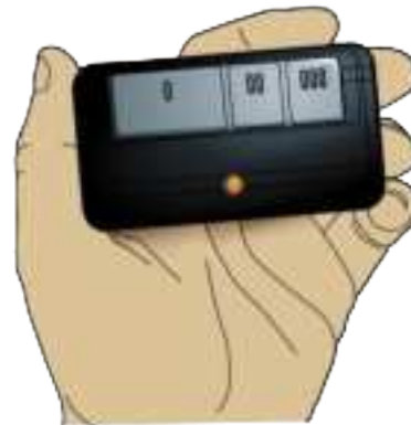
3-Button Remote Control programmed for OPEN, CLOSE, and STOP
