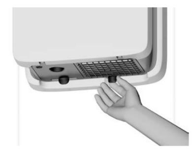
It is advisable to clean the filter every time the ffuussTM hand dryer receives external maintenance. It is recommended the HEPA Filter is replaced 12 monthly or more frequently in high use situations.
