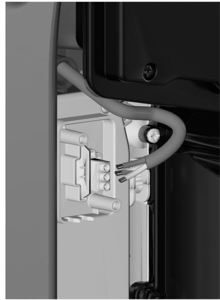
Once the cable has been passed through the hole, connect each end to its respective terminal, placing each one in the right path and then close the box.
