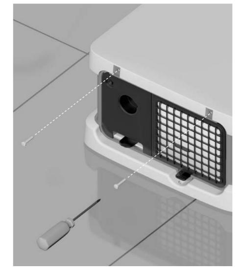
Take the ffuussTM hand dryer from its packaging and open the front cover to install the electricity cable. Open the cover of the connector box which is where the cable to the network will be installed.
