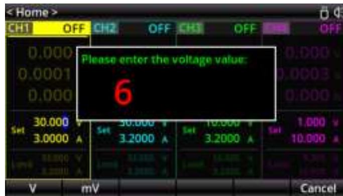
Figure 4-1 Keypad Editing for Voltage
