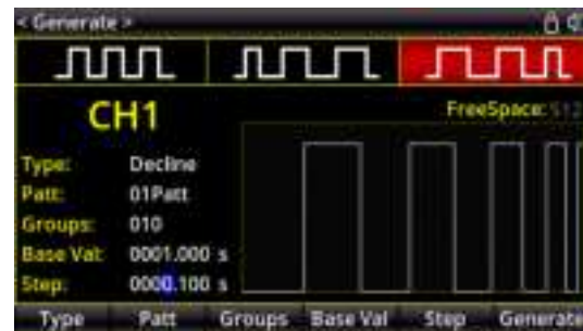
Figure 9-3 Monotonically Increasing Time Template Figure 9-4 Monotonically Decreasing Time Template
