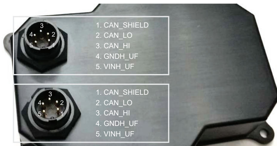
Figure 3 - Connector Pinout
