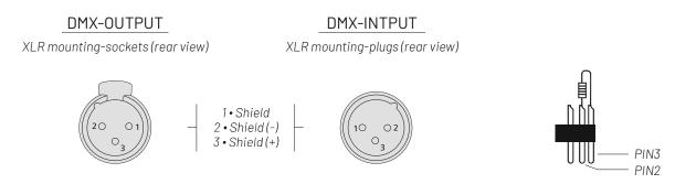
When using standard DMX512 control signal, the last device's output interface must be connected to a DMX plug. This plug is putting a 120 ohm resistance between "canon" plug's 2 pin and 3 pin. Showing as below pic. Sticking this plug into the last device's signal output interface, it will avoid the interference during the process of signal transmission.
