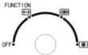
**Function knob 2;** includes settings for OFF, Rotisserie function on, Rotisserie function and Convection fan on and Convection fan on.
