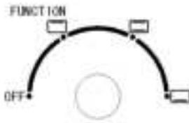
**Function knob 1;** includes settings for OFF, Upper element on, Upper and Lower elements on and Lower element on.
