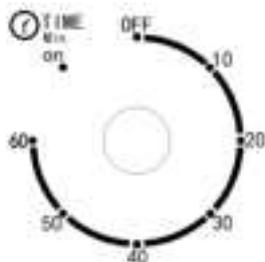
**TIMER knob;** Controls oven on duration. Includes settings for "on" allowing for continuous operation, OFF and variable control to 60 minutes.
