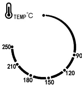
**Thermostat knob;** includes settings for OFF and variable control for oven temperature from 90 to 250 degreesC.
