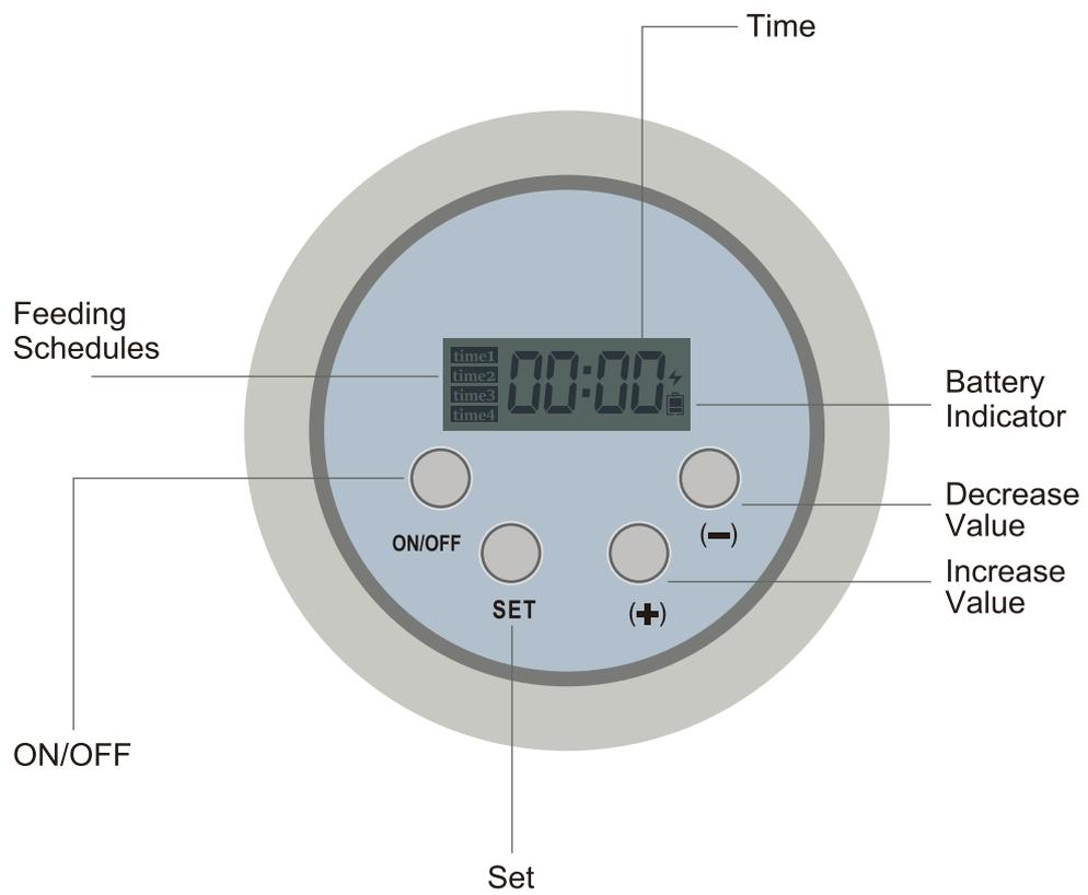
The feeder remembers your personalized settings every time and uses a 24 hour clock system, which be divided into 4 times per 24 hours. The default timing of **time1** is 06:00, **time2** is 11:00, **time3** is 16:00, **time4** is 21:00.
