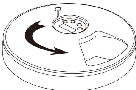
**2** Turn the lid counterclockwise by hand to open the top cover
