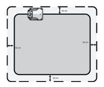
The recommended distance between two pegs is about 80 cm in straight lines, and less in tight curves. Note that the peas' hook and wire slit always faces the outside of the boundary. Within a short time the cable will be covered with grass. Since the voltage is only 32 V, there is no risk of electric shock. Make sure that the hook of the peg and the opening for the cable always face the demarcated.
