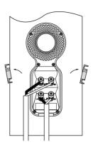
Ensure that the positive terminals on the speaker (marked + and coloured red) are connected to the positive output terminal on the amplifier and the negative terminals on the speaker (marked – and coloured black) are connected to the negative output terminal on the amplifier. Incorrect connection can result in poor imaging and loss of bass.
