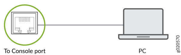
Figure 15: Connect an ACX710 Router Directly to a Management Console
