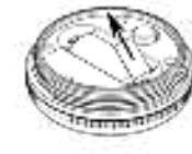
Remove the Face Plate from the sensor by turning the Face Plate counter-clockwise and pull the battery tab to start the pairing process.
