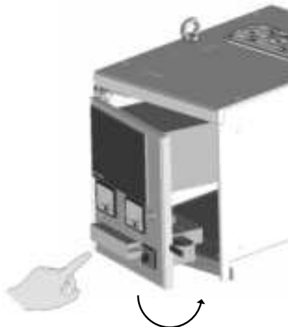
Figure 3-17: Closing top unit
