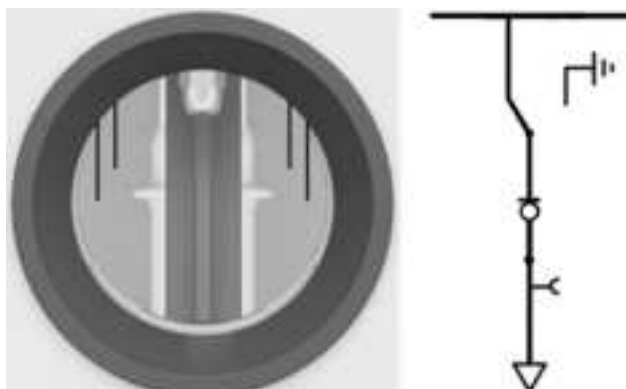
Figure 4-3: Service position - (VI closed and change-over in busbar position)
