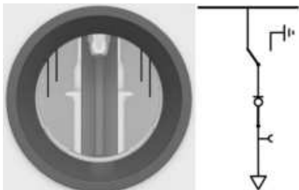
Figure 4-8: Service position - change-over switch in the busbar position and VI closed
