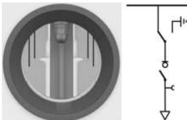
Figure 4-4: Open position (VI open and change-over in busbar position)
