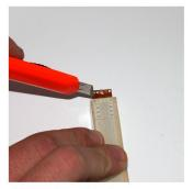
Use a sharp blade to carefully cut back the TPU housing 3/8" without cutting the PC Board.
