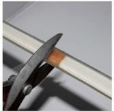
Cut the ribbon on the cut line closest to your re-connection point.
