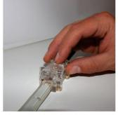
Unscrew the allen bolts on the connector, slide in the ribbon completely and tighten the allen bolts.
