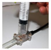
Apply silicon gel to the small hole in the back of the connector until overflow is seen on the top two holes.
