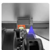
Use mechanical level to ensure ultrasonic beams are pointing downwards at the truck side frame.
