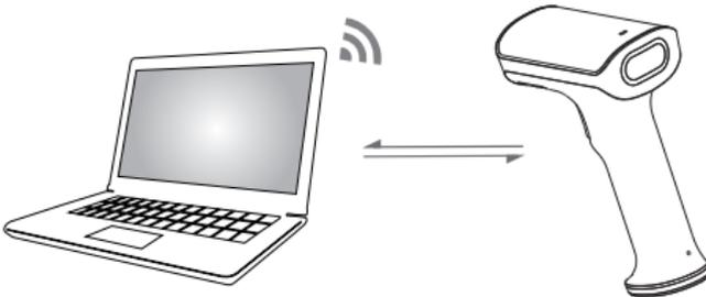
The scanner is shut up by pressing the scanning button, and be connected it to the host devices through Bluetooth. The green light indicates that it is connected and can be used normally.
