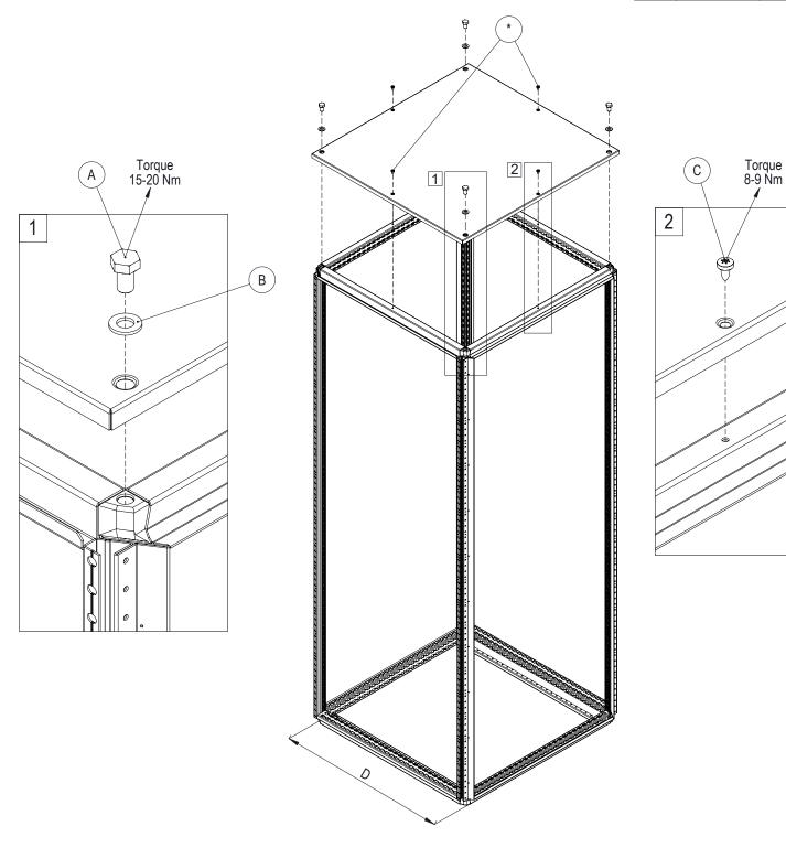
$<sup>^{\</sup>star}$  - Used on enclosures 800 mm deep. \*\* - Torque value for first tightening. For following tightening, torque value recomended is 4-5 Nm.
