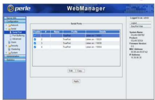
Select the port that is connected to the VDCP controller/automation device and click on Edit...
