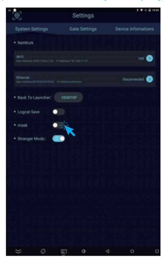
2 ) Stranger mode(Turn on stranger mode, the device will flash red status light for unregistered face users to show early warning! Don't open the door!)
