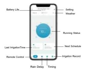
Press the "Timing" button and then the "+", you can set "Normal Schedule" or "Cycle/soak" watering program.
