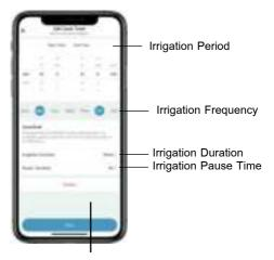
Whole Schedule: During 10:00AM to 10:00PM, the timer will cycle watering program for 5 mins and stop for 6hrs. The timer will watering at 10:00-10:05AM and 4:05-4:10PM.
