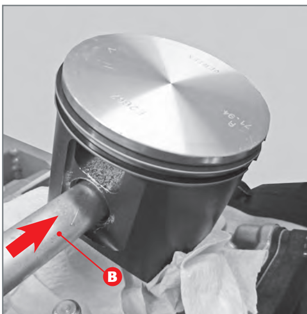
Removal of pin bolt.
