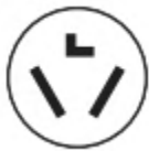
3-wire receptacle (10-30R)
