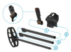
Release the locking lever located at the bottom of the handle. Then, push the handle into the upper rod. Next, press down the locking lever to secure it in place. Insert the armrest to the button of upper rod, use a Phillips screwdriver to tighten it securely.
