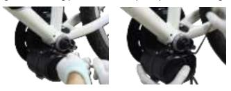
8) Tighten the fixing block screws completely with the hexagonal wrench.
