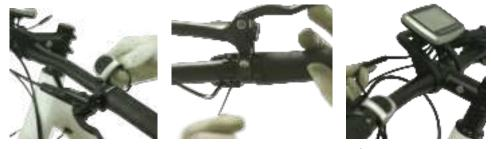
4) Throttle Installation: Loosen the screw on the throttle then fix the throttle on the right handle by tightening the screw completely. Finally, connect the throttle wire to the middle socket at the back of display.
