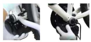
9) Assemble the cranks: Tighten the crank screws with the M8 hexagonal wrench (locking torque: 35-40N.m).
