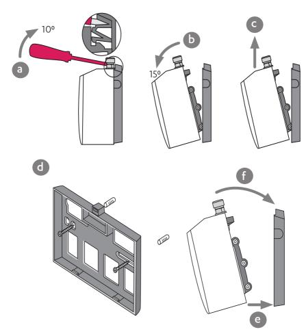
**Note** Take care not to break the clips when removing or installing the Booster.
