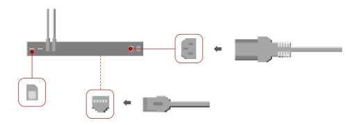
^ Cellular is Enabled in LSP-enabled devices. The sim must be able to connect via the default APN 'Broadband' in the event the appliance is unable to connect via the network interface.
