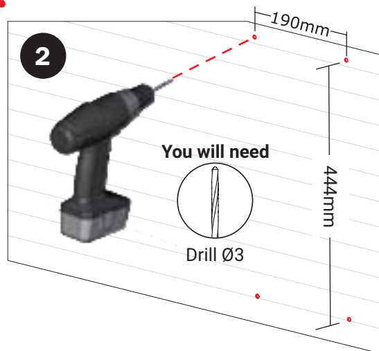
Fig.2: Make holes with Ø3 drill.
