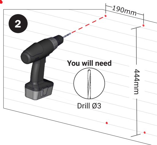
Fig.2: Make holes with Ø3 drill.
