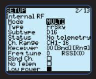
Frequency tuning. Certain protocols require tuning for optimal performance. In some cases, tuning is required in order for the protocol to bind. Frequency Tuning is specific to each MULTI-Module, and is due to very small variations in the RF components.
