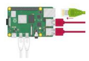
8. Plug the power supply into a socket and then connect it to your Raspberry Pi's USB power port.
