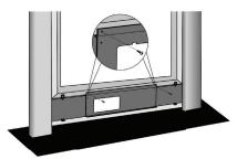
6 Using one pointed screw, install the Security tracket to the window.
