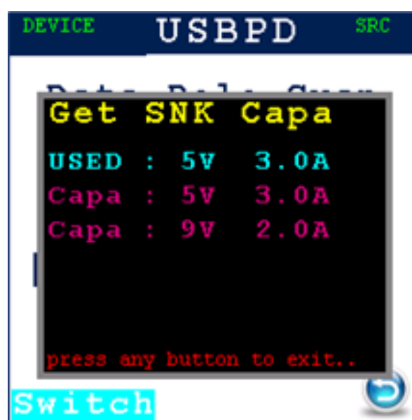
Figure 17. USBPD Sink capabilities
