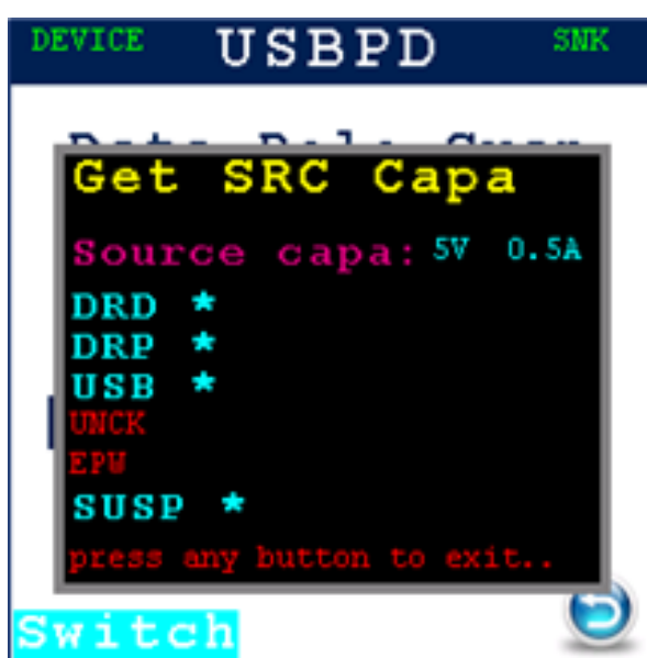
Figure 16. USBPD Source capabilities
