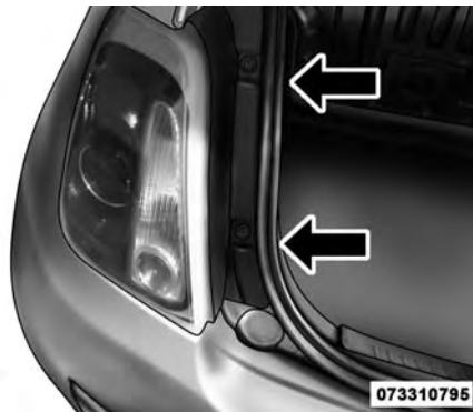
Tail Lamp Assembly Screws
