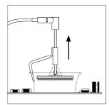
The component lifts off automatically when the solder melts.
