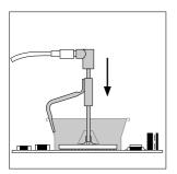
Position the extractor with the appropriate suction cup and press the suction button.
