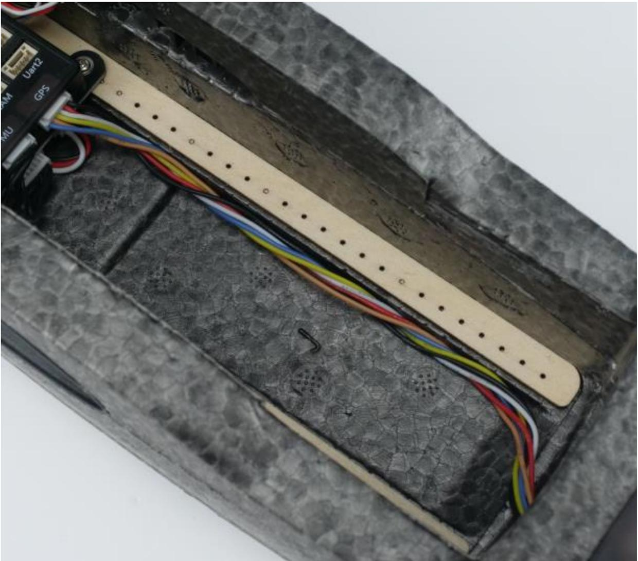
n. Place the battery mount onto the wooden rail, align the screw holes and secure it with 4pcs of 2x6 screw.
