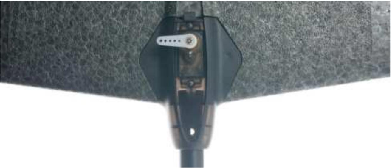
e. Align the vertical stabilizer onto the clip of the horizontal stabilizer as shown below and install it.
