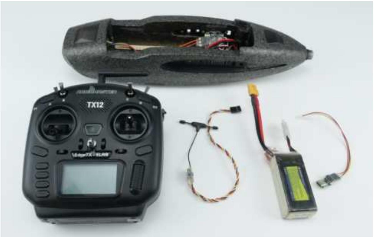
Connect your preferred receiver to the RC-In port of the FX-405 Flight Controller.
