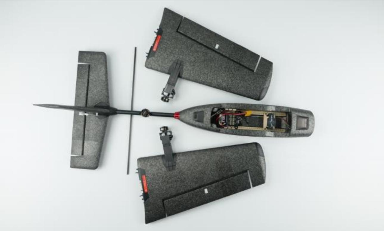
y. Slot the carbon rod into the main wing\
