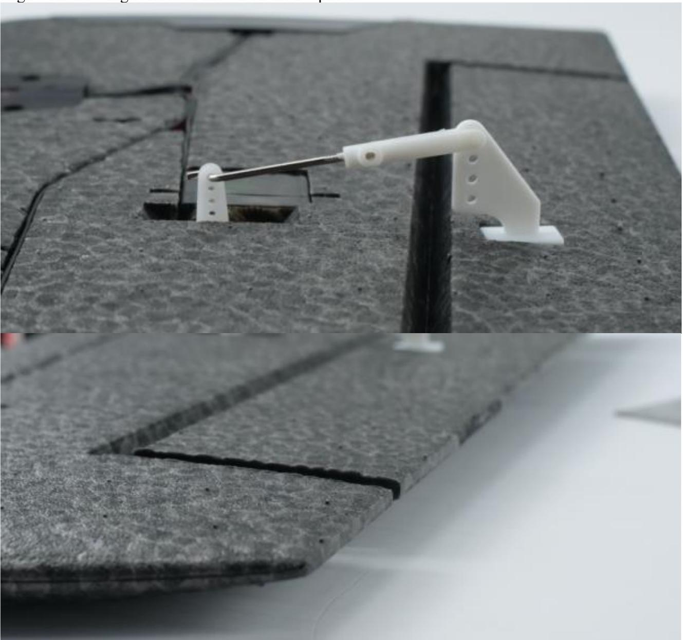
t. Install control horn onto the elevator and secure it with the latch
