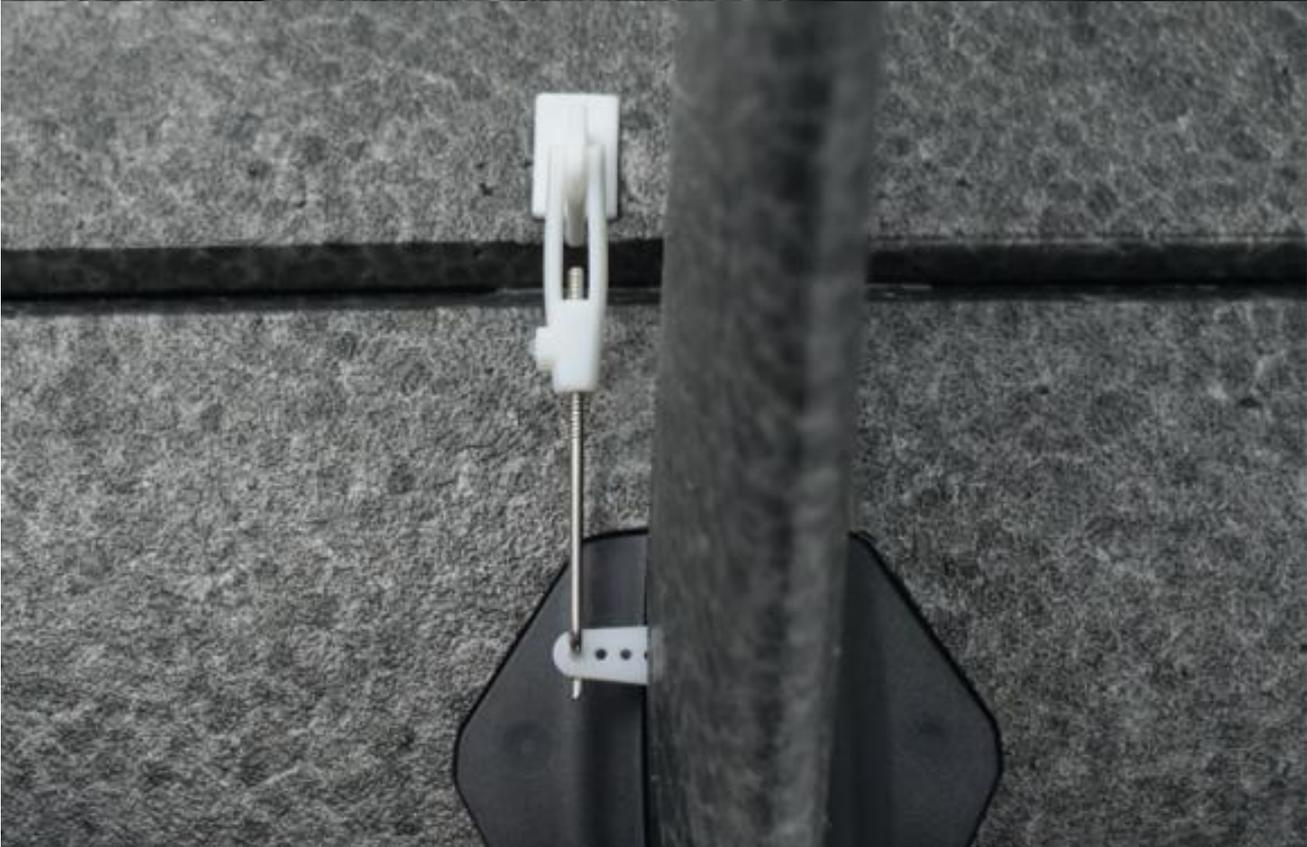
v. Ensure that the elevator is parallel to the horizontal stabilizer by adjusting the linkage length
