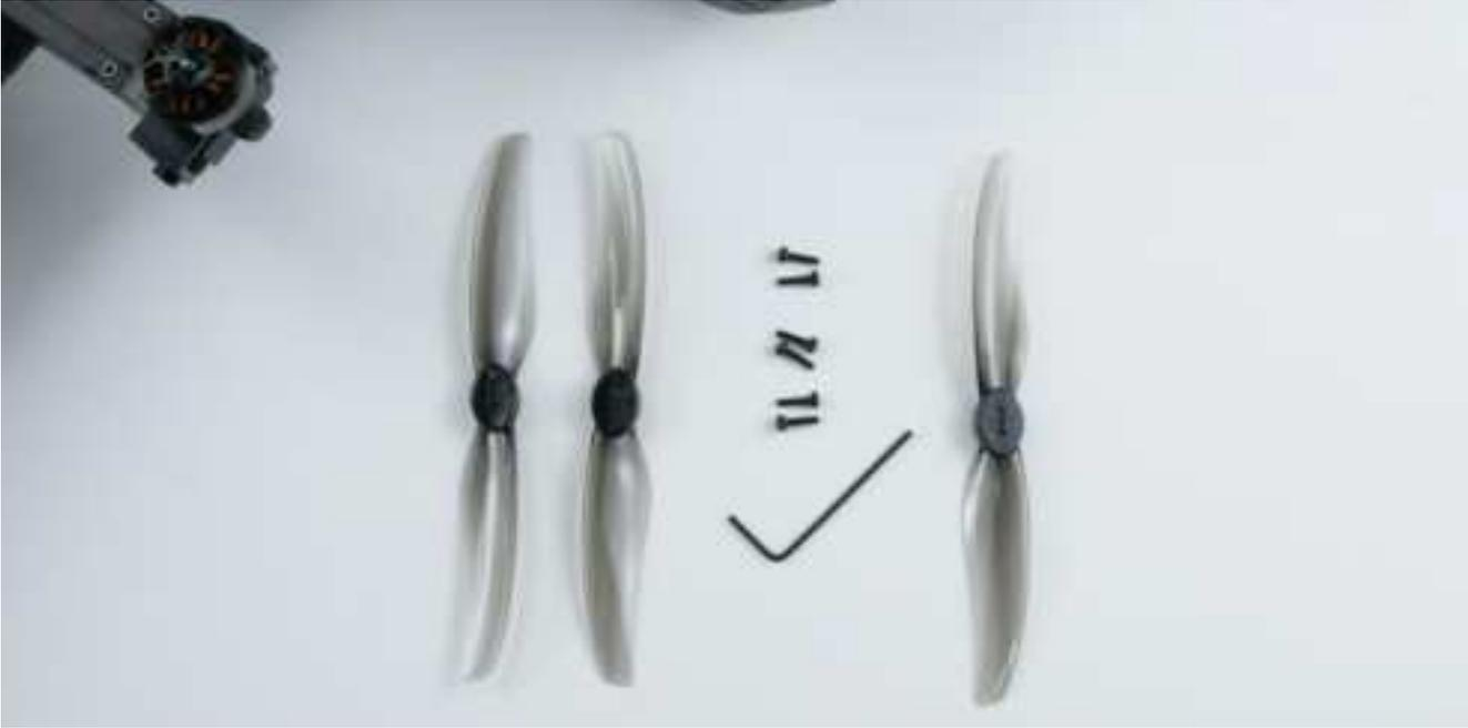
ah. Secure the propeller onto the motor with the screws. Observe orientation of the propeller.
