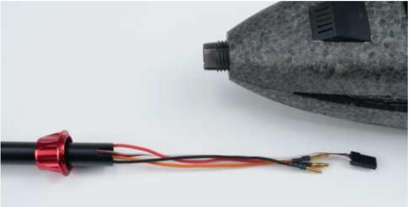
I. Slot in the wires into the fuselage together with the tail boom and secure it with the nut. Do not need to over tighten the nut as long as it's not loose.
