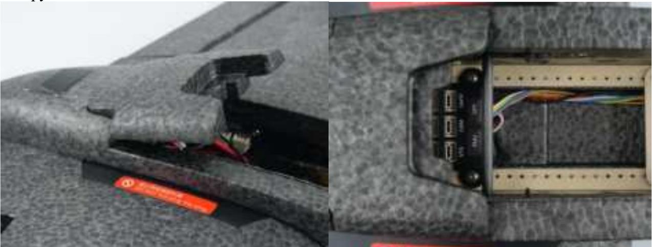
ae. Now slide the canopy with the hatch towards the front, gently press the latch onto the carbon rod to secure it onto the fuselage.
