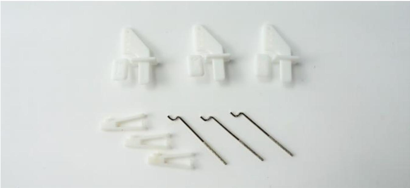
p. After installing the steel linkage into the latch, place it in the opening of a vernier caliper, the end to end length should be 46mm. If you do not have a vernier caliper, you may use a ruler. Repeat the same thing for the other 2 linkages.
