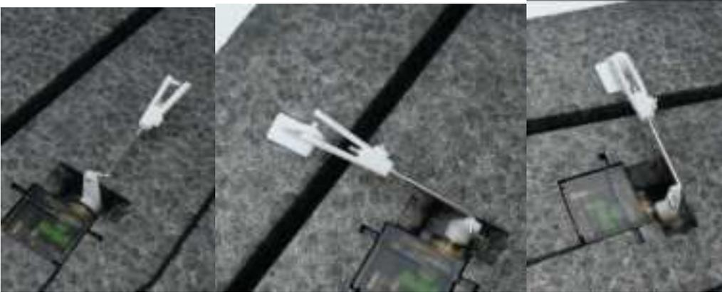
s. The servo horn angle should be parallel to the wing surface. With the servo centered (best when it's powered), you may adjust the linkage length accordingly to ensure that the control surface is align with the wing surface as shown on the 2<sup>nd</sup> photo
