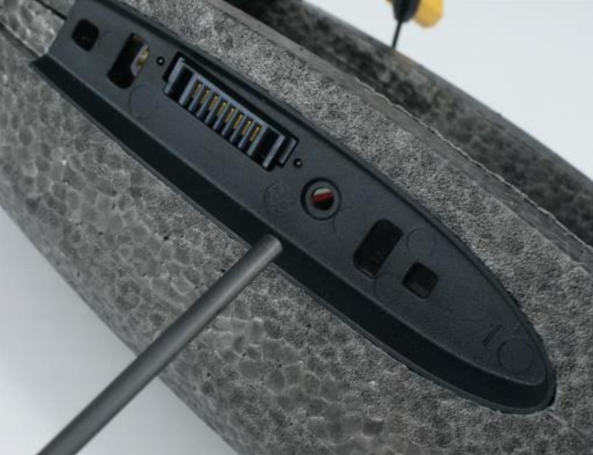
z. Carefully attach the main wing onto the fuselage and ensure that it's properly clipped onto.
