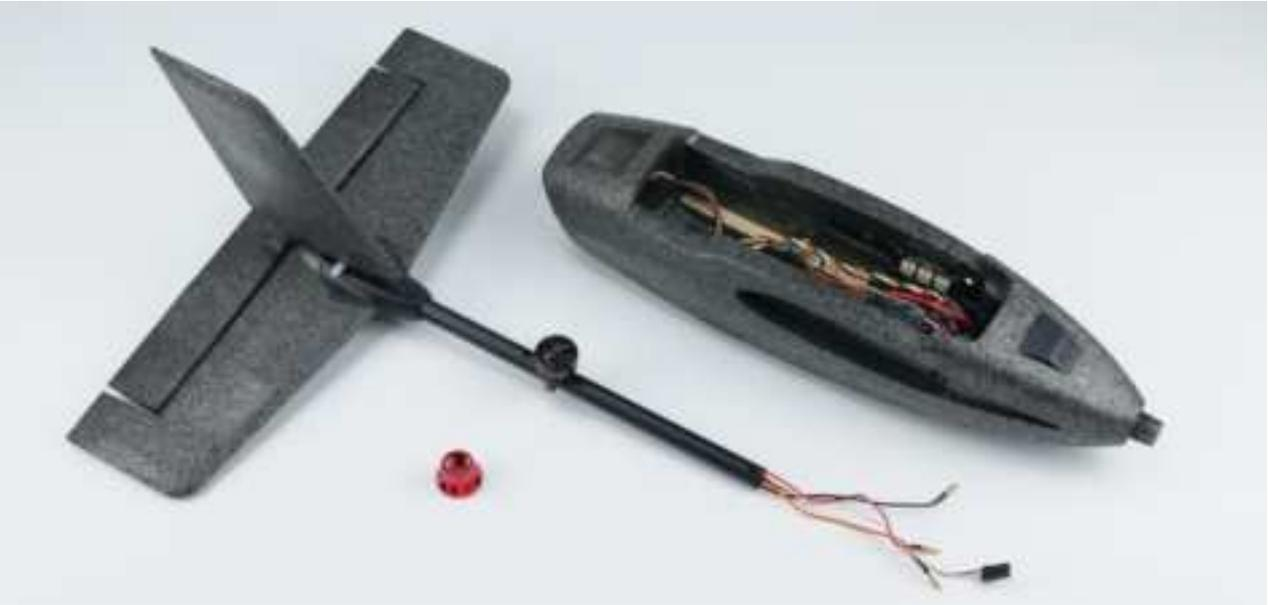
h. Slot the red color nut onto the tail boom first, observe the direction as shown below
