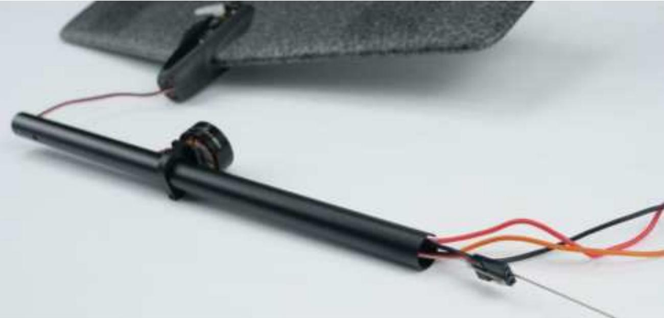
c. Observe the U Shape cut on the tail boom and align it to the stop inside the horizontal stabilizer mount.
