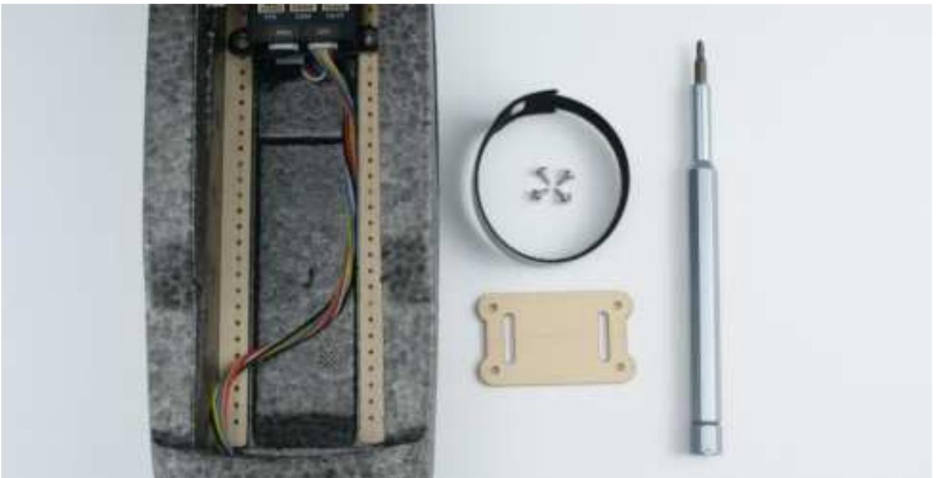
m. Slot the battery strap through the battery mount, organize the wires to one side to prevent the wires getting squashed
