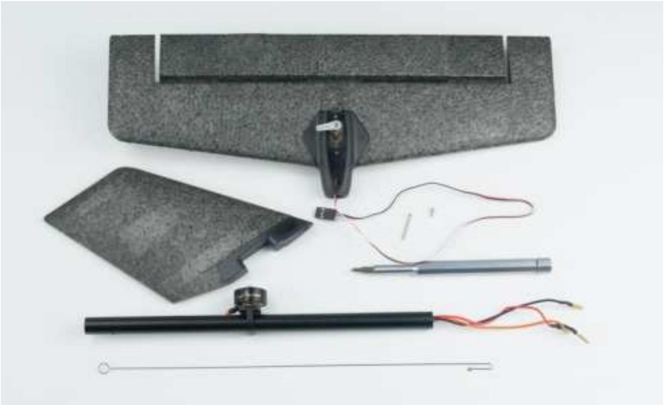
b. Using the provided guide wire, pull the servo connector through from one end of the tail boom to the other end of the tail boom
