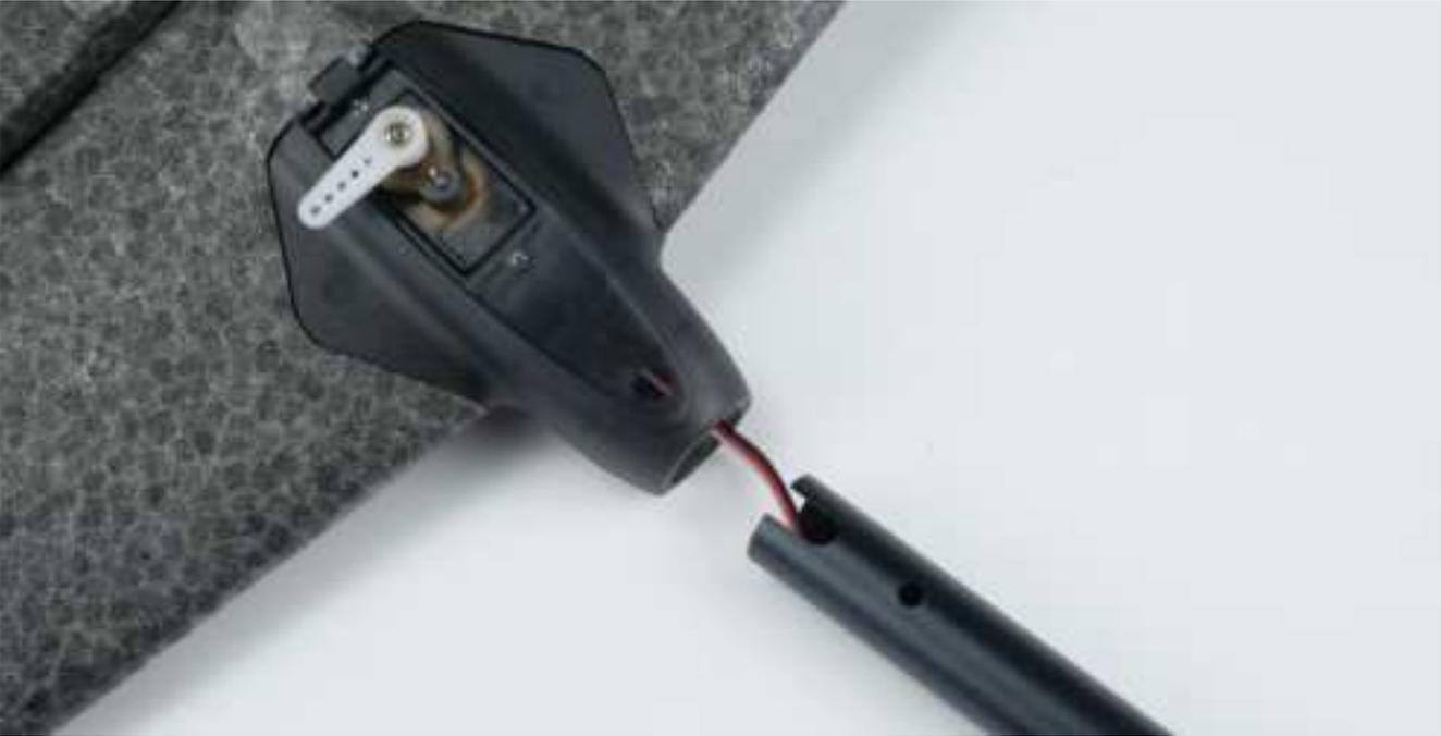
d. After inserting the tail boom, ensure the U shape cut is centered and is not pushing onto any wires. If installed correctly, the hole is clearly see through and the servo wire is visible as well.
