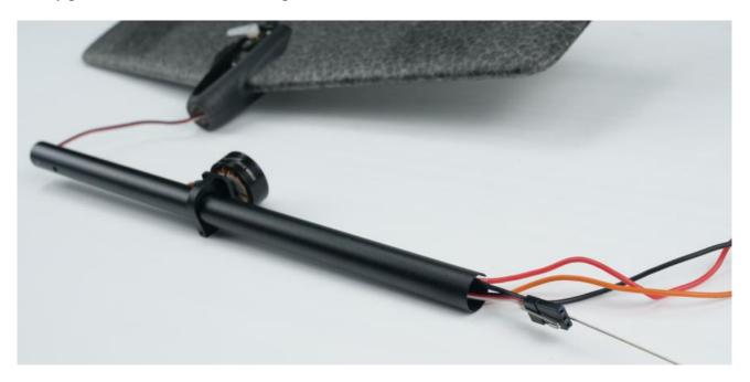
c. Observe the U Shape cut on the tail boom and align it to the stop inside the horizontal stabilizer mount.
