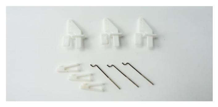
p. After installing the steel linkage into the latch, place it in the opening of a vernier caliper, the end to end length should be 46mm. If you do not have a vernier caliper, you may use a ruler. Repeat the same thing for the other 2 linkages.
