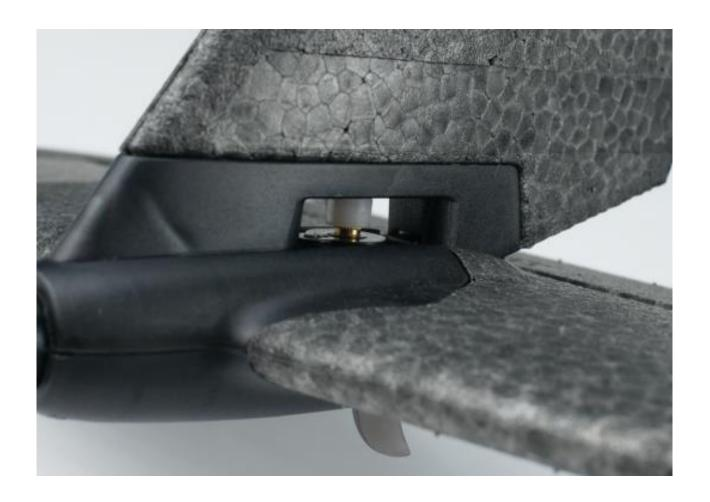
f. Rotate to the other side and install the corresponding screws according to the marking on the mount.
