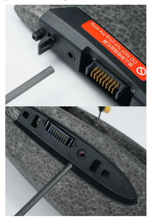
z. Carefully atach the main wing onto the fuselage and ensure that it's properly clipped onto. \*Do not attach or detach the main wing while it's powered as this can damage the electronics
