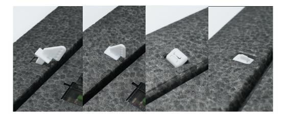
r. Slot the steel linkage into the hole on the servo horn that is furthest away from the center, then secure the other end onto the control horn.
