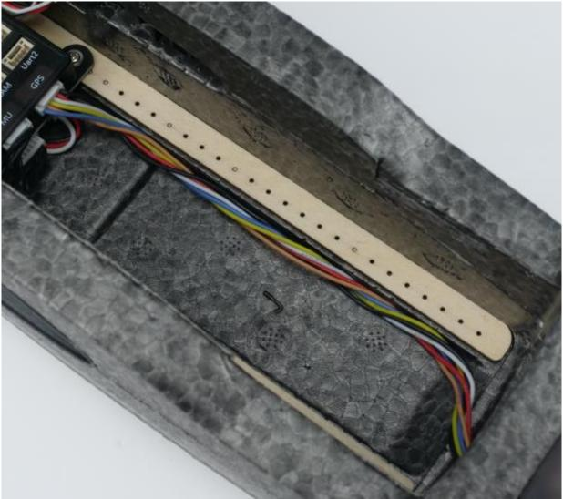
n. Place the battery mount onto the wooden rail, align the screw holes and secure it with 4pcs of 2x6 screw.
