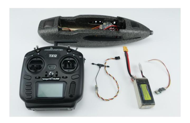
Connect your preferred receiver to the RC-In port of the FX-405 Flight Controller. \*Note the Ground, 5V & Signal line.
