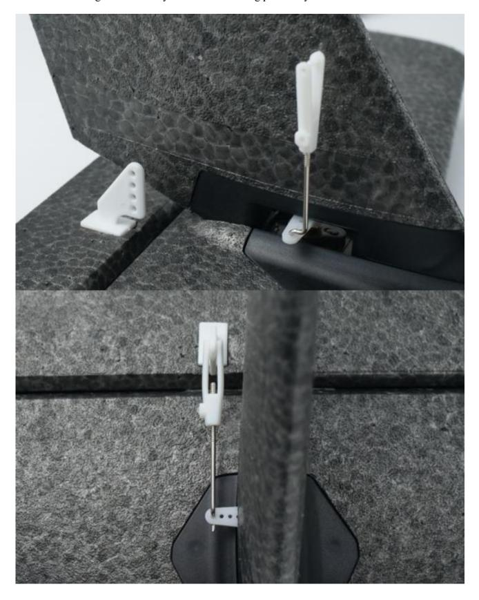
v. Ensure that the elevator is parallel to the horizontal stabilizer by adjusting the linkage length
