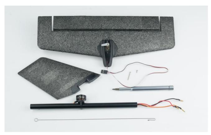
b. Using the provided guide wire, pull the servo connector through from one end of the tail boom to the other end of the tail boom
