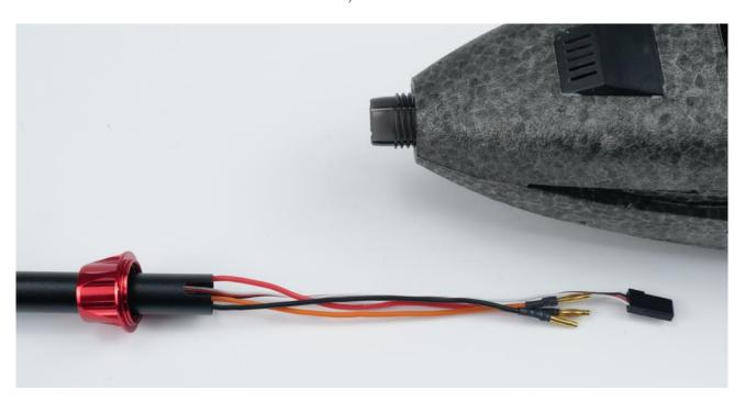
I. Slot in the wires into the fuselage together with the tail boom and secure it with the nut. Do not need to over tighten the nut as long as it's not loose.
