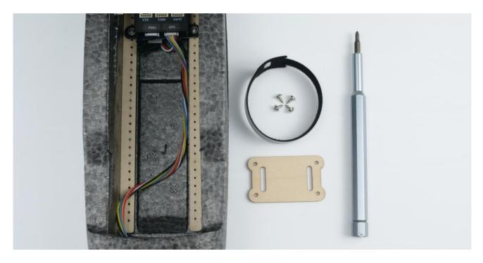
m. Slot the battery strap through the battery mount, organize the wires to one side to prevent the wires getting squashed
