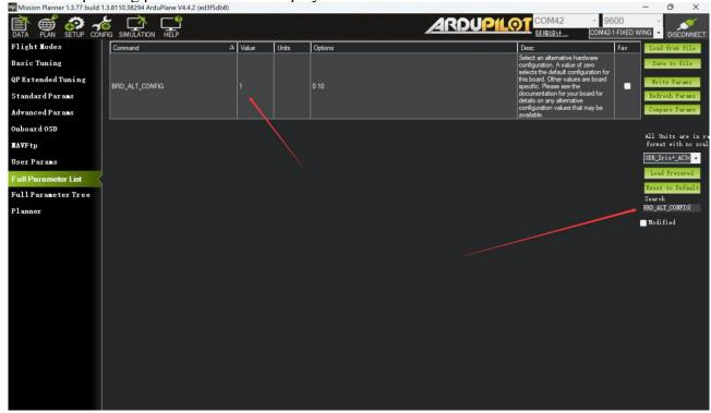
Change the "Value" from "1" to "0", then click "Write Params" to write the changes to the flight controller. Click "Ok" to confirm.
