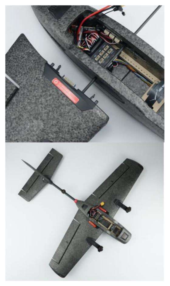
ab. Installing latch of the canopy
