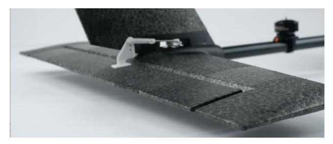
x. Installing wings onto the main body/fuselage
