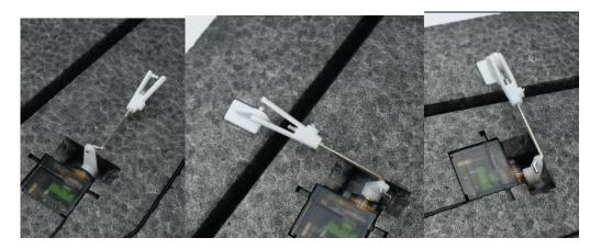
s. The servo horn angle should be parallel to the wing surface. With the servo centered(best when it's powered), you may adjust the linkage length accordingly to ensure that the control surface is align with the wing surface as shown on the  $2^{nd}$  photo
