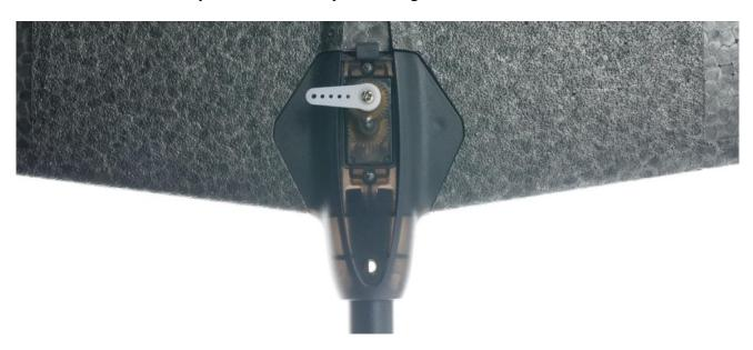
e. Align the vertical stabilizer onto the clip of the horizontal stabilizer as shown below and install it.
