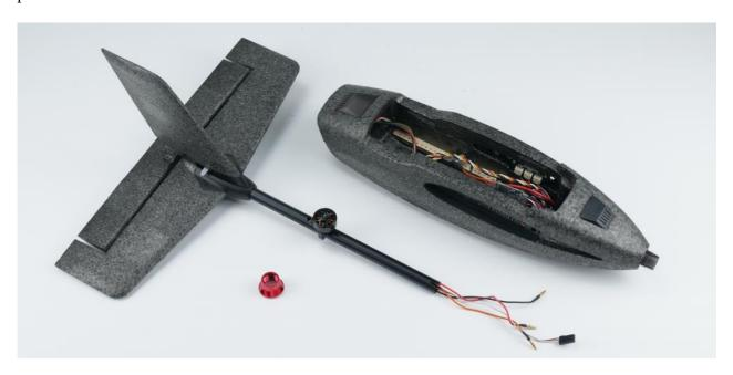
h. Slot the red color nut onto the tail boom first, observe the direction as shown below
