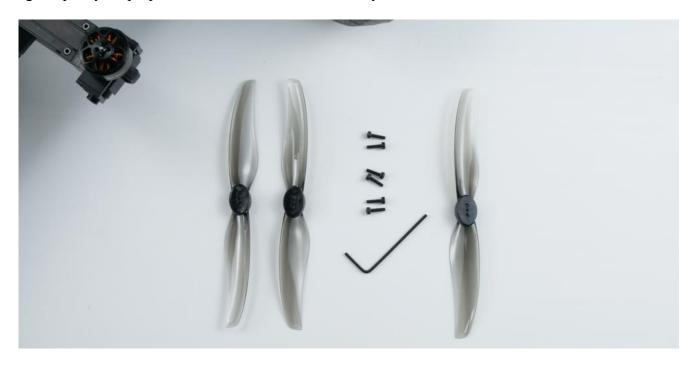
ah. Secure the propeller onto the motor with the screws. Observe orientation of the propeller.
