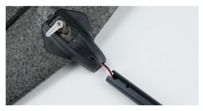
d. After inserting the tail boom, ensure the U shape cut is centered and is not pushing onto any wires. If installed correctly, the hole is clearly see through and the servo wire is visible as well.
