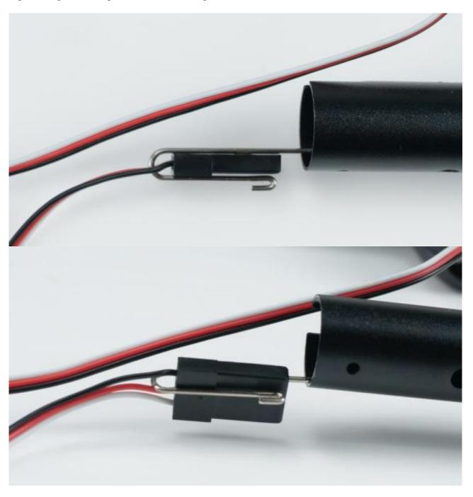
Gently pull the servo connector through the tail boom to the other end as shown
