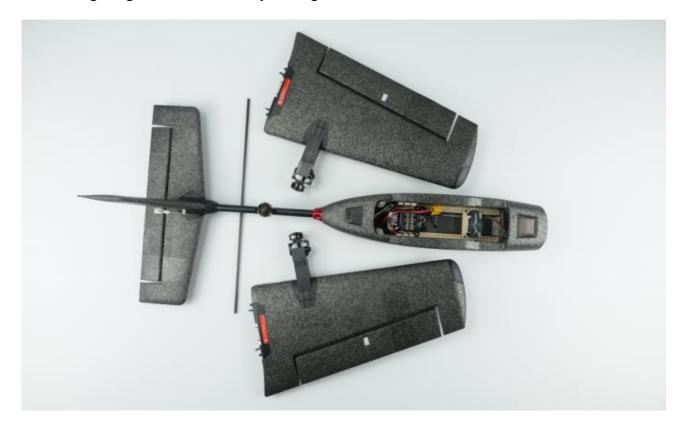
y. Slot the carbon rod into the main wing\
