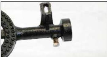
4. Install burner assemblies with two fiat head screws, washers, lockwashers, and nuts.
