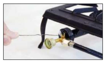
4. Check each flame port opening in the diffuser to make sure there is no blockage from food or other debris.
