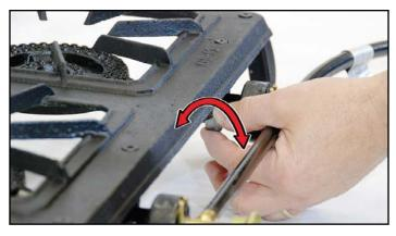
7. If the burner flame does not burn blue, check the burner venturi for obstructions. Dirt daubers, spiders, and other insects will build nests blocking air and gas flow.
