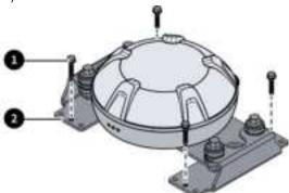
Method 2: Use the 3M stickers ❷ to fix the GNSS receiver bracket ❶.
