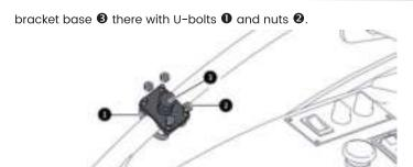
Step 2: Fix the bracket base • on the back of the terminal holder bracket • with screws and place in and fix the terminal •. Rotate the handle of the adapter bracket • counterclockwise to loosen the ball socket, and then install the ball joint on the back of the terminal into the ball socket of the bracket.
