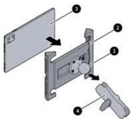
Step 3: Install the ball joint ② of the base into the other ball socket of the adapter bracket ①, and rotate the handle clockwise to firmly fix the terminal.
