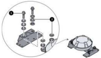
Step 2: Use the tapping screws or 3M stickers, whichever suitable, to fix the GNSS receiver on the top.
